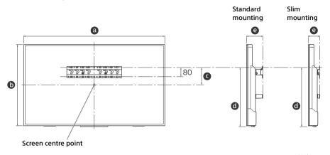
Unit: mm Screen **Display dimensions** centre Length for mounting dimension **Model Name** KDa 0 G 0 **e** Standard Slim mounting mounting 65X7500D 1,463 852 26 458 142 100 55X7000D 1,245 730 86 458 141 99 448 99 49X7000D 1,107 651 116 141
