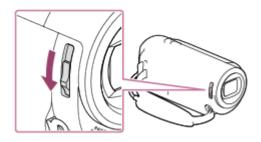
2. Open the LCD monitor of this product and turn the power on.
