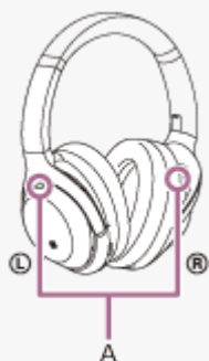
A: Noise canceling function microphone (external)
